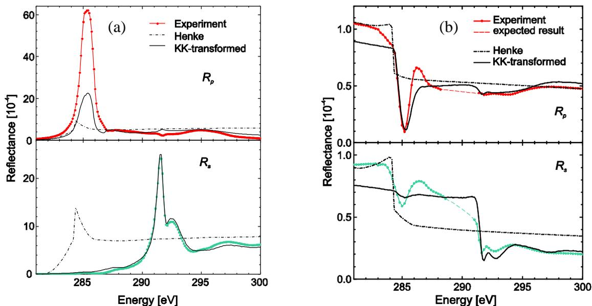
Fig. 2. Simulation of the measured reflectance for (a) HOPG and (b) graphene on copper using KK-transformed data (solid) and Henke data (dash-dot). In (b), between 288 eV and 291 eV, the reflectance is unknown due to the insensitivity of the measurement – the expected result is shown instead as dashed line.
