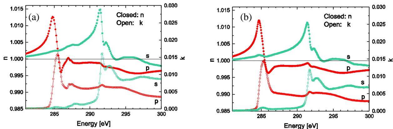
Fig. 1. RI experimental optical constant  $n$  and deduced extinction coefficient  $k$  of (a) HOPG and (b) graphene.
