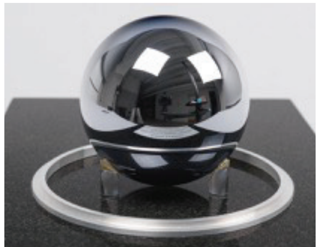
One kilogram silicon sphere. Source: [3].
