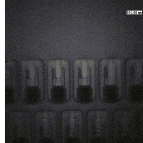
Top view of bubble formation in a Memjet chip
