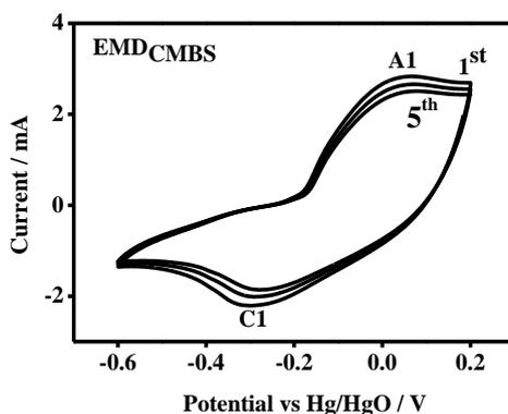
Fig. 4. Cyclic voltammetry plot of  $\text{EMD}_{\text{CMBS}}$  with cycling at a scan rate of  $0.2 \text{ mV s}^{-1}$ .
