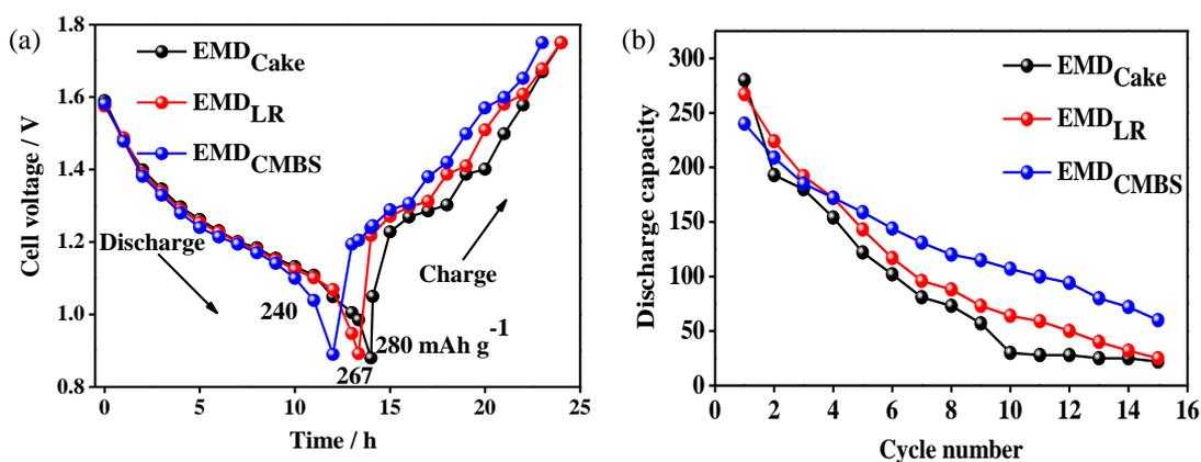
Fig. 3. (a) The first discharge-charge profile and (b) discharge capacity vs cycling behaviour of Zn/EMD cells obtained from different sources.
