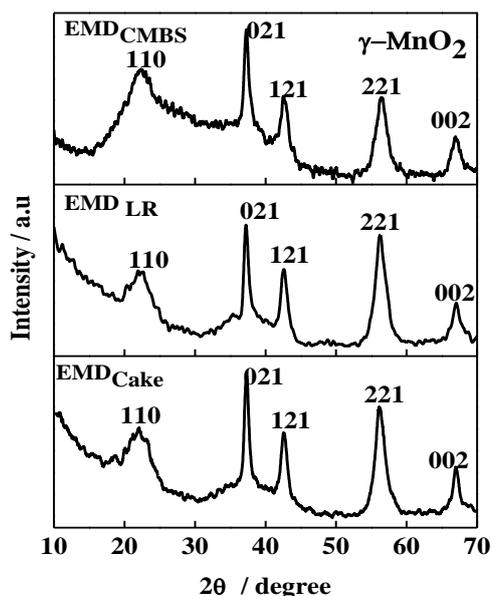
Fig. 1. XRD patterns of EMD samples synthesized from different sources.
