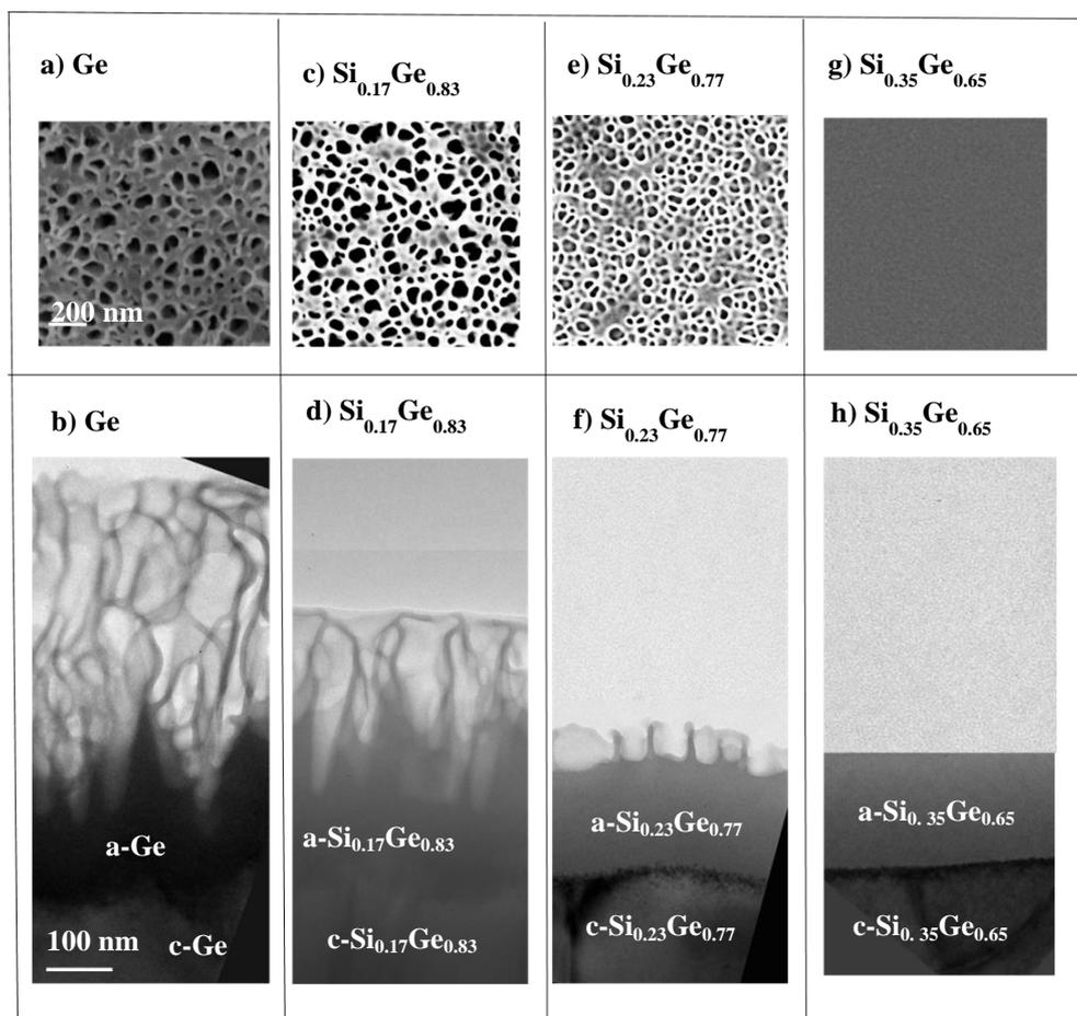
Fig. 1. PVSEM and XTEM images of Ge<sup>+</sup> implanted Si<sub>1-x</sub>Ge<sub>x</sub> alloys with different Ge stoichiometry for the same fluence of  $2 \times 10^{17}$  ions/cm<sup>2</sup> (a) (b) in Ge, (c) (d) in Si<sub>0.17</sub>Ge<sub>0.83</sub>, (e) (f) in Si<sub>0.23</sub>Ge<sub>0.77</sub>, (g) (h) in Si<sub>0.35</sub>Ge<sub>0.65</sub>. The scale bar is the same for all PVSEM and XTEM images, respectively.
