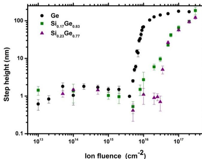
Fig. 4. Volumetric swelling as a function of ion fluence for Si<sub>1-x</sub>Ge<sub>x</sub> alloys with different Ge content at 23°C irradiation.
