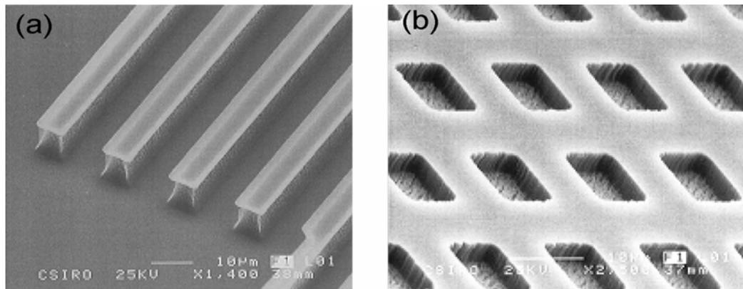
Figure 4. Microstructures etched using CF<sub>4</sub>/O<sub>2</sub>.
