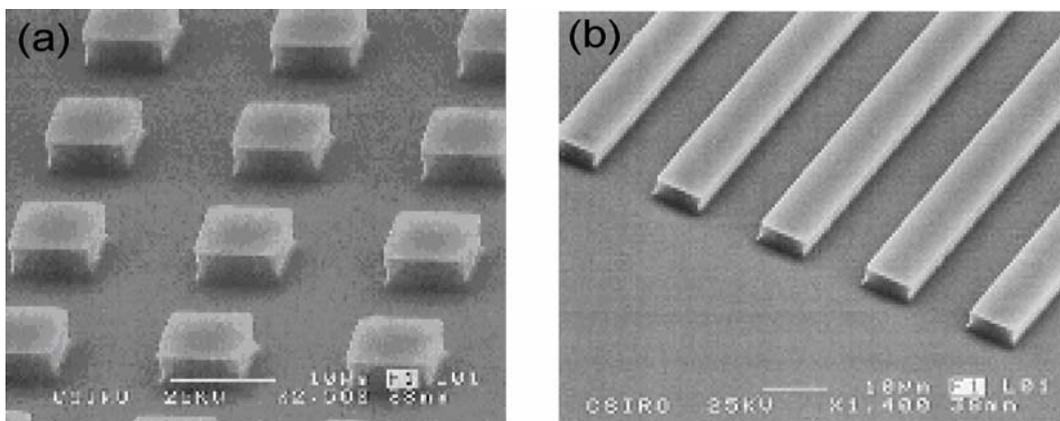
Figure 3. Smooth surfaces and near-vertical sidewalls observed on SOI arrays of  $10 \times 10 \mu\text{m}^2$  pillars and  $6 \mu\text{m}$  waveguides etched using  $\text{CF}_4/\text{Ar}$  mixture.
