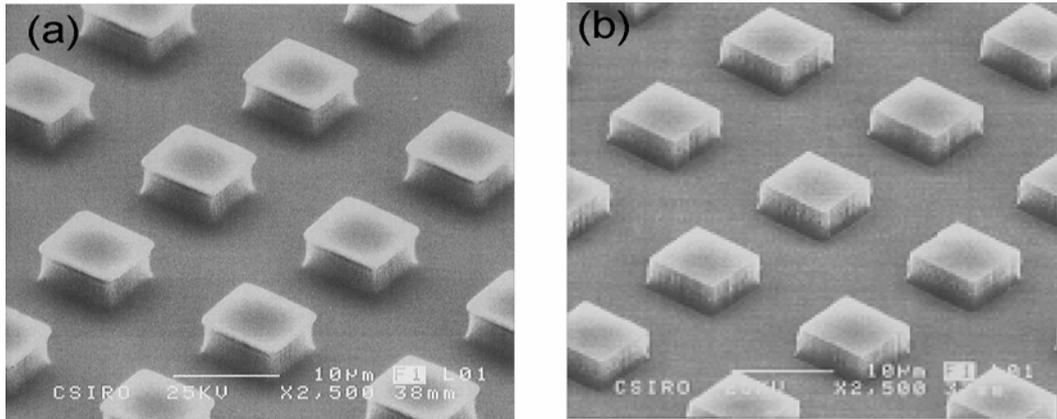
Figure 2. Array of  $10 \times 10 \times 4 \mu\text{m}^3$  pillars on Si etched at  $\text{CF}_4$  pressure (a) 10 Pa and (b) 3 Pa.
