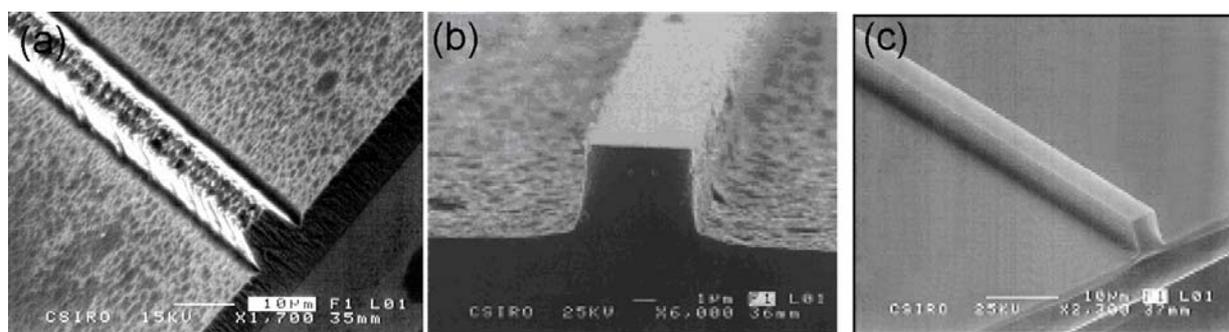
Figure 1. Silicon rib waveguides etched using (a) resist mask, and (b, c) Ni-Cr masks.
