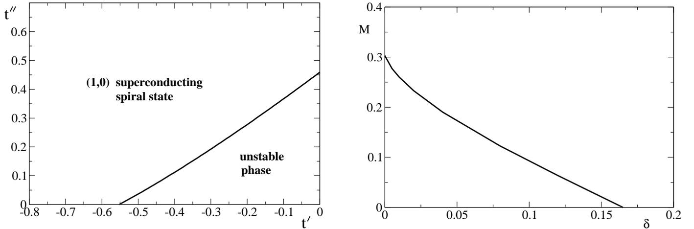
FIG. 2: The left figure shows phase diagram of the  $t - t' - t'' - J$  model at  $t = 3.1$  and small doping,  $\delta \ll 1$ . The bottom right corner corresponds to the pure  $t - J$  model,  $t' = t'' = 0$ . The top left corner corresponds to parameters from Ref.[26], Eq. (2). The region of stability of the superconducting (1,0) spiral phase is shown. The right figure shows on-site magnetization in the (1,0) spiral versus doping for  $t = 3.1$ ,  $t' = -0.8$ , and  $t'' = 0.7$ .
