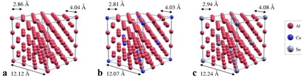
Figure 2. Equilibrium geometries calculated using the FLAPW method. (a) Pure aluminium. (b) Aluminium with copper impurities. (c) Aluminium with tin impurities.
