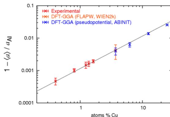
Figure 3. Numerical and experimental [9] results for the mean lattice parameter  $\langle a \rangle$  of solid solutions of copper in aluminium.
