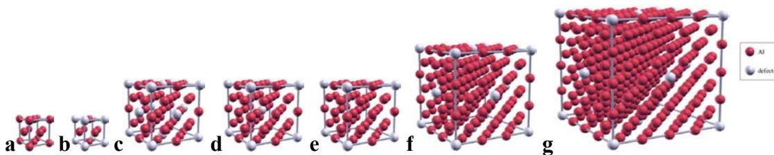
Figure 1. Supercells used to model substitutional defects in face-centred cubic aluminium. Defect concentrations (number of defects per lattice site) are (a) 0, (b) 1:4, (c) 1:8, (d) 1:16, (e) 1:32, (f) 1:27, (g) 1:64.
