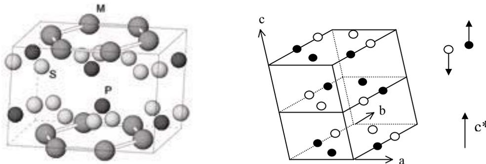
Fig. 1a) Crystallographic structure of MPS<sub>3</sub> and b) the previously accepted magnetic structure of FePS<sub>3</sub> [1]. Arrows represent magnetic moment directions parallel to *c*\*.
