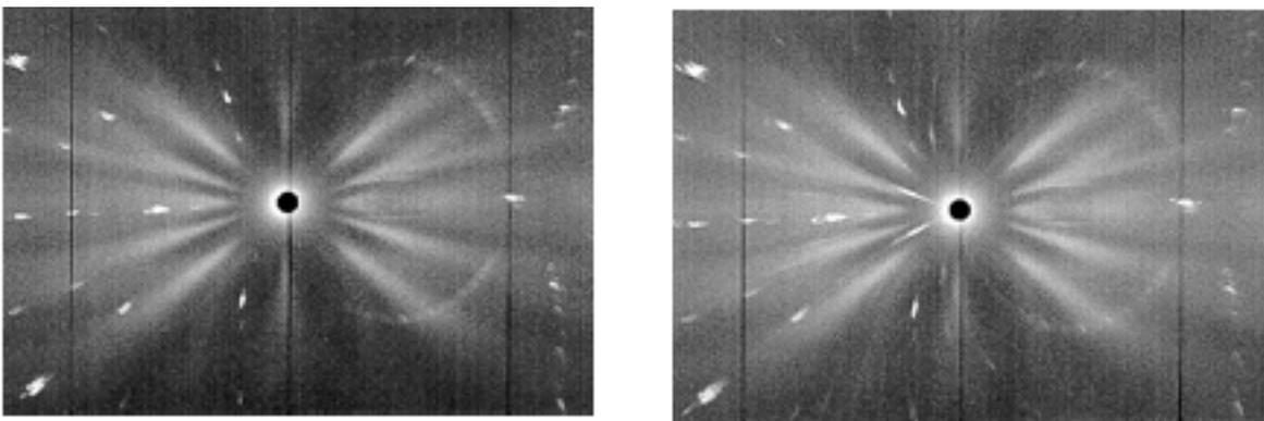
Fig. 2 Laue diffraction patterns from VIVALDI at 140 K (left) and 5 K (right).
