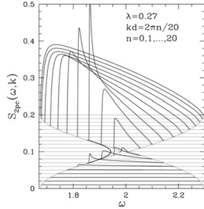
Fig. 4. A 'sliced' view of the structure factor for the 2-particle continuum versus energy for different momenta  $kd = 2\pi n/20$ ,  $n = 1, \dots, 20$  at  $\lambda = 0.27$ . The solid line is the dispersion relation for the bound state  $T_1$ . Note how the structure factor peaks where the bound state enters the continuum.
