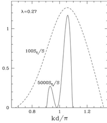
Fig. 3. Relative spectral weights of the triplet bound states  $T_1$  and  $T_2$  at  $\lambda = 0.27$ . Note the dip in the middle for  $T_2$ .
