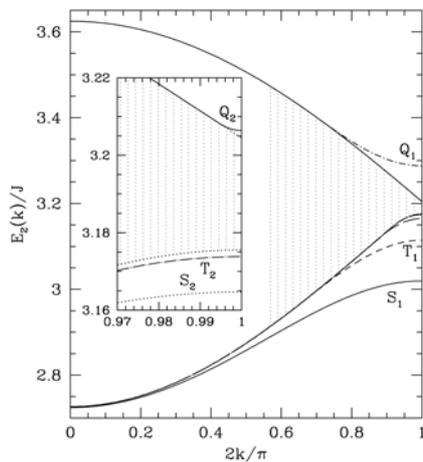
Fig. 1. Dispersion diagram for 2-particle states showing singlet (S) and triplet (T) bound states, plus quintet (Q) ‘antibound’ states. The inset shows a second pair of bound states below the continuum.
