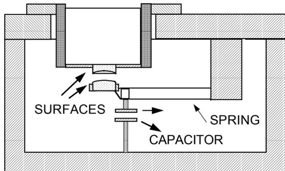
Fig. 1. Schematic diagram of surface force apparatus with capacitance stage. The lower moving surface is attached to a double cantilever spring, thereby ensuring that the surfaces remain parallel when the spring is deflected. The top plate of the capacitor is fixed to the moving cantilever head, the bottom is stationary.
