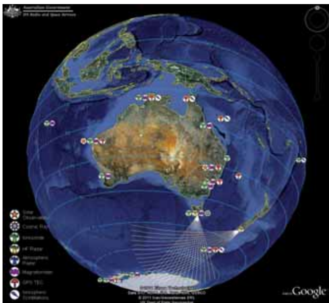
Fig. 1. The IPSNET ground-based multi-sensor array covering about one-eighth of the Earth's surface. The array is grouped by priority region for new sites, maintenance, upgrade and replacement. The highest priority mid-latitude region is further grouped into continental Australia and surrounding islands. Sensor types are indicated in the key.
