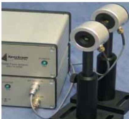
Warsash Scientific is pleased to announce a near-IR addition to the revolutionary Delta Radiometer / Joulemeter series from Spectrum Detector Inc. The Delta NIR Joulemeter provides near-IR spectral response from 0.9 to 1.7  $\mu\text{m}$ , while also offering numerous performance advantages unique to the Delta Series of joulemeters and radiometers.
